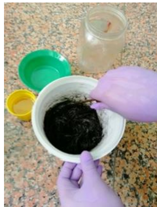
FIGURE (3) Hand Lay-up
