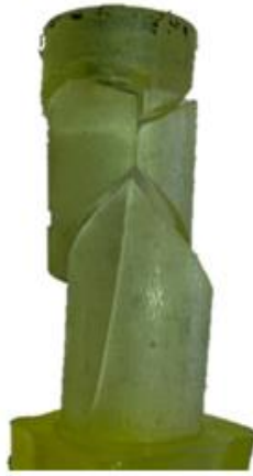
Fig. 5: Epoxy tube failure after burst pressure test.
