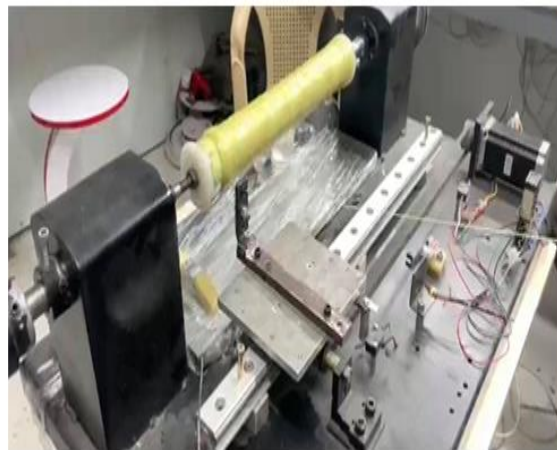
Fig. 1: The filament wound machine construction and elements.
