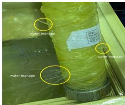
Fig. 6: the water leakage results from burst pressure test.
