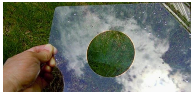
Figure (15) shows a glass plate in which the circular area has been coated with an anti-reflective nano-coating, while the rest of the plate has not been coated. 17
