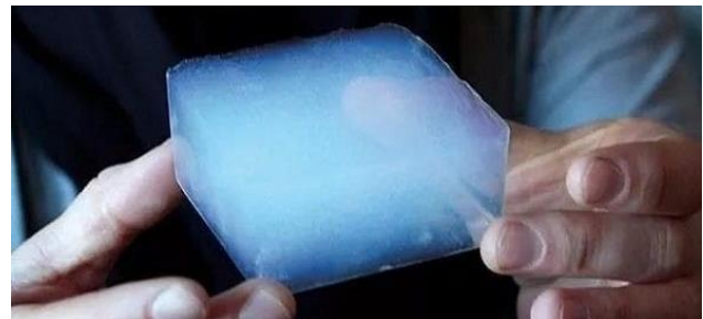
Figure (20) shows the transparent material of the aerogels. 27
